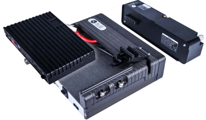
VoyagerMCAT showing the Mini-CATAPAN and Voyager 1 battery module removed
