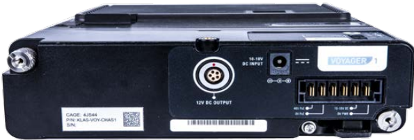
Rear view showing the Voyager 1 battery module attached to the VoyagerMCAT
