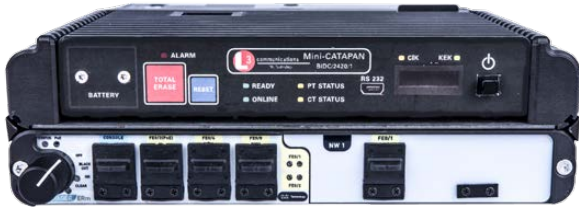
Front view showing Voyager m-Series module with Mini-CATAPAN on top
