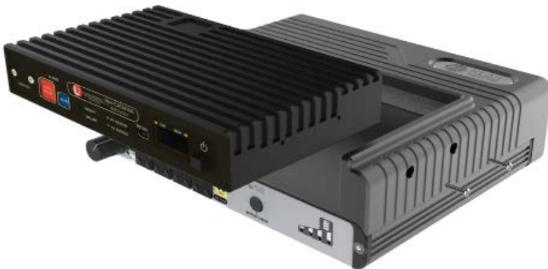
Mini-CATAPAN can be removed by releasing 4 screws in the side of the unit
